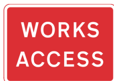
Example signage – Temporary Construction Traffic Signage – P7301 from DfT Traffic Signs Manual Chapter 8 part 3
